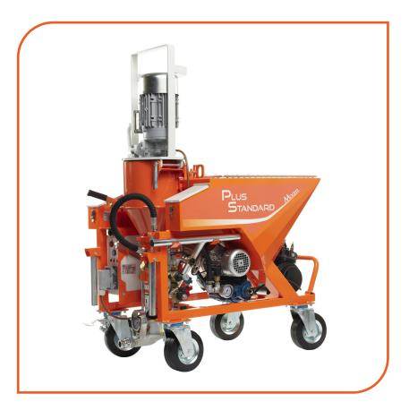
Mixer Plus Top and Mixer Plus Standard are three-phase (400 V) continuous mixing pumps, ideal for spraying pre-mixed surface coatings containing lime, cement, finishing compounds, fillers, coloured compounds, adhesives, screeds, etc. and any product compatible with the mechanical spraying.
